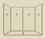
A x4 14<sup>3</sup>/<sub>4</sub>" (374mm) W x 37" (940mm) H 1" (25mm) panel thickness
