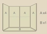
14<sup>3/</sup>4" (374mm) W x 37" (940mm) H 1" (25mm) panel thickness
