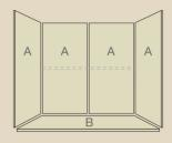
A x4 14<sup>3</sup>/<sub>4</sub>" (374mm) W x 37" (940mm) H 1" (25mm) panel thickness
